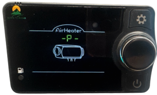
The LCD Displays “P” when its Priming.
