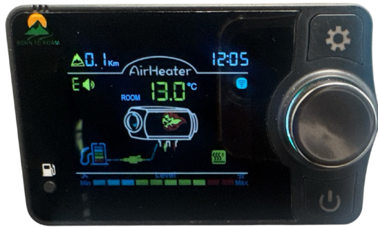
The flame icon confirms the glow plug is lit.
